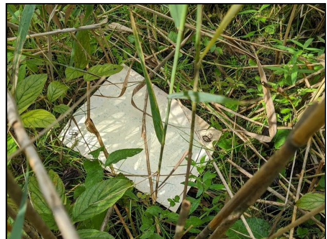
To gauge the amount of herbicide reaching the understory plant zone from the ARGO, sheets of heavy white paper were randomly placed on the ground. This allowed us to see individual droplets of herbicide.
