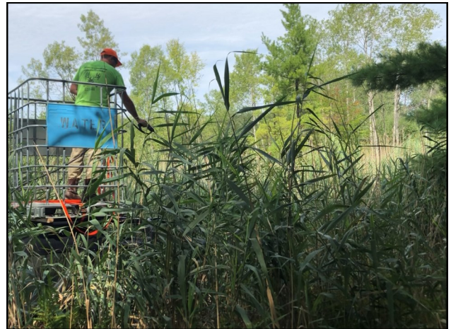
A roof mounted cage on the ARGO allowed herbicide to be sprayed from above to get good coverage on the actively growing areas of common reed.
